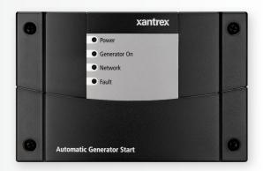
The Xanbus Automatic Generator Start (AGS) is a control module that automatically activate a generator to provide Freedom SW Inverter/Charger\* with power to recharge depleted batteries or assist with heavy loads. Having an AGS in your system means that power is available and battery banks are charged automatically so you do not have to spend time monitoring power consumption.
