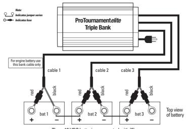
Three 12 VDC batteries connected with (2) series jumpers for a 36 VDC trolling motor
