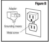
Use of an adapter is not allowed in Canada. If a grounding type receptacle is not available, do not use this appliance until the proper GFCI protected outlet is installed by a qualified electrician.
