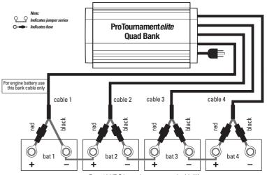
Four 12 VDC batteries connected with (3) series jumpers for a 48 VDC propulsion system
